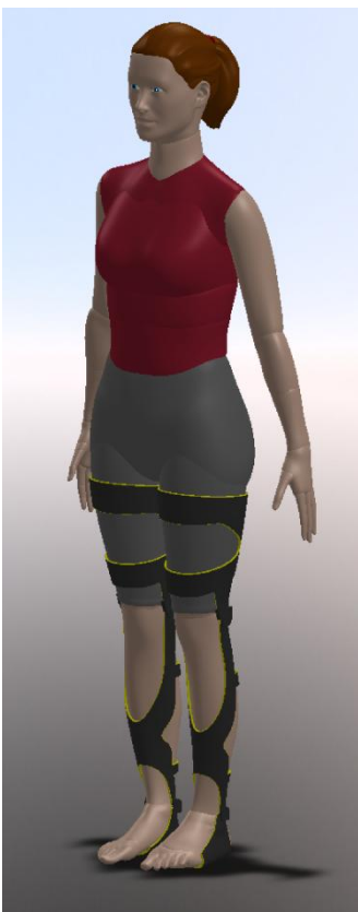
Figure 4: A Female Mannequin used to test a proposed carbon fiber exoskeleton design.
