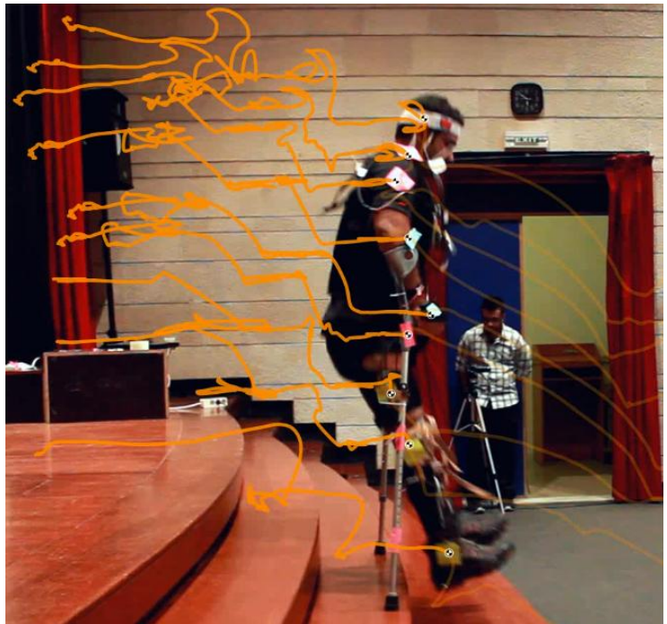
Figure 1: Photo of Michael during an experiment at LAU. The motion and acceleration of his limbs are being tracked and recorded.
